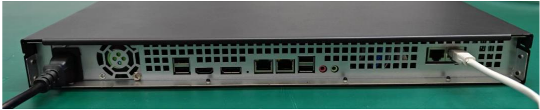
1U edge all-in-one machine connection mode
